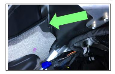
11. Install the three push darts (6) securing the console.
