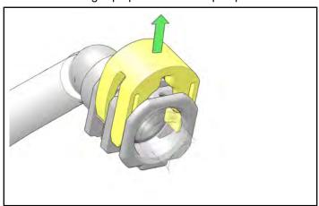
6. Remove quick connect from the fuel fitting.
