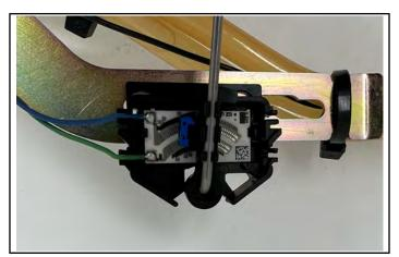
Level Sender Card Photo - Clearly show level sender card clip is fully clipped in and shows blue dot.
