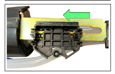
8. Install the level sender card into the card holder. Verify both wires are secured in the retention features and both tabs are securing the sender card.
