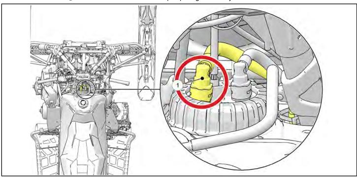
2. The fuel return line should route down the front of the fuel tank. The return line should be secured in the foam block ② and connect to the corresponding line ③ from the fuel rail in the locations shown below.
