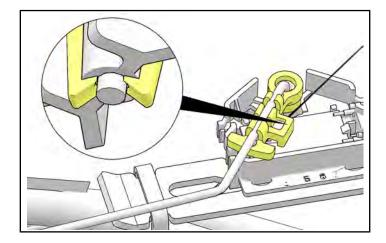
11. Verify both metal tabs of the wiper arm are not damaged and maintain contact with the card through the full range of motion.
