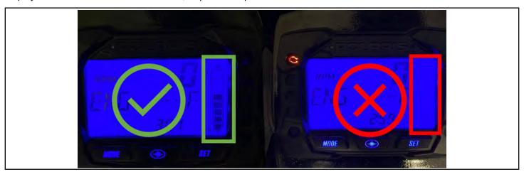
The PIDD will not show a fuel level indicator if the wiper arm was not correctly installed. Note that other system gauges may display in place of the fuel level indicator. Make sure that the gauge displayed is a fuel level indicator.
