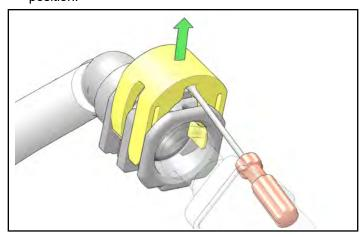
3. Remove quick connect from the fuel fitting.
