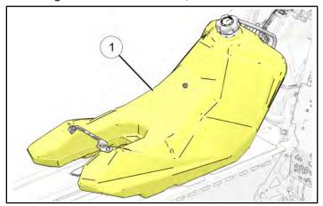
3. Install a new front tank mount fastener ② (Short M6 fastener provided) securing the fuel tank bracket to the fuel tank. Torque fastener to specification.
