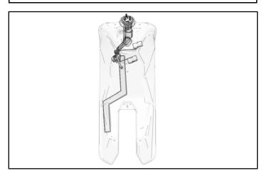
4. Align the fuel pump flange assembly index marks with the arrow on the fuel tank ②.
