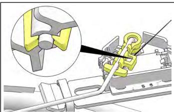
Remove the level sender card by carefully releasing the locking tabs. Do not damage the wires when removing the level sending card.
