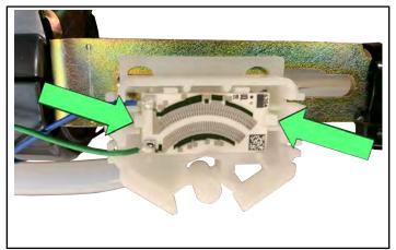
Remove the card holder by releasing the locking tab on the back of the card holder while pushing in the direction shown.
