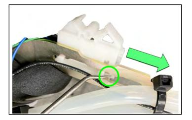
Install the new level sender card holder by sliding into
