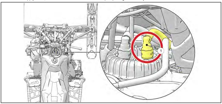
2. The fuel supply line should route down the front of the fuel tank. The supply line should be secured in the foam block ② and connect to the corresponding line ③ from the fuel rail in the locations shown below.
