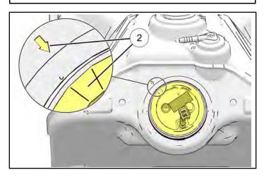
5. Spray the PFA gasket with isopropyl alcohol to assist with PFA nut install. With the help of an assistant holding the fuel tank, use the PFA nut socket and PFA hold fixture to torque the nut ③ to specification.
