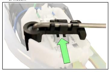
12. Inspect the entire ground wire for damage, corrosion, or loose connections. If any damage is found, STOP and contact Polaris Technical Service.
