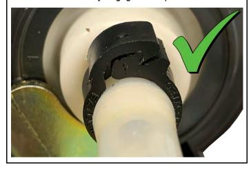
4. Remove the float arm as an assembly by releasing the two tabs on the back side of the fuel level sender.
