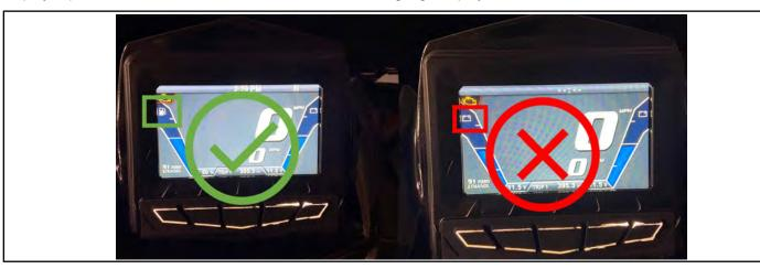
The Polaris 7S Digital Display will show low fuel if the wiper arm was not correctly installed. In order to properly verify fuel gauge operation, ensure the vehicle has enough fuel for the display to show fuel level. Once fuel has been added, if the display still shows low fuel, inspect the wiper arm for correct installation.
