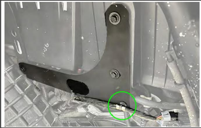
16. Route the fuel pressure sensor harness underneath and back through the hole in the bracket. Connect it to the sensor until a click is heard, and engage the red secondary retaining tab by pushing it towards the sensor.
