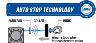
Auto Stop technology protects and extends the life of your winch by automatically stopping the winch at the end of pull to prevent over-spooling. While plowing, it prevents the plow frame from bending by stopping the winch once the plow has been lifted.
